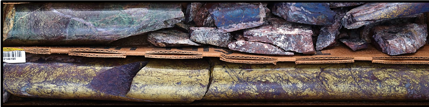
High-grade hypogene enrichment mineralization responsible for 1-2% Cu at top of porphyry system.
