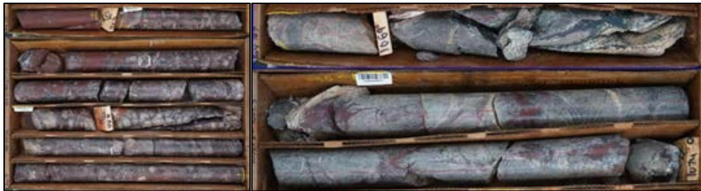
Drill hole 24-12 illustrating the transition from Jurassic cover, through oxidized leach cap, and then into the high-grade hypogene enrichment mineralization at depth (bornite-chalcocite).
