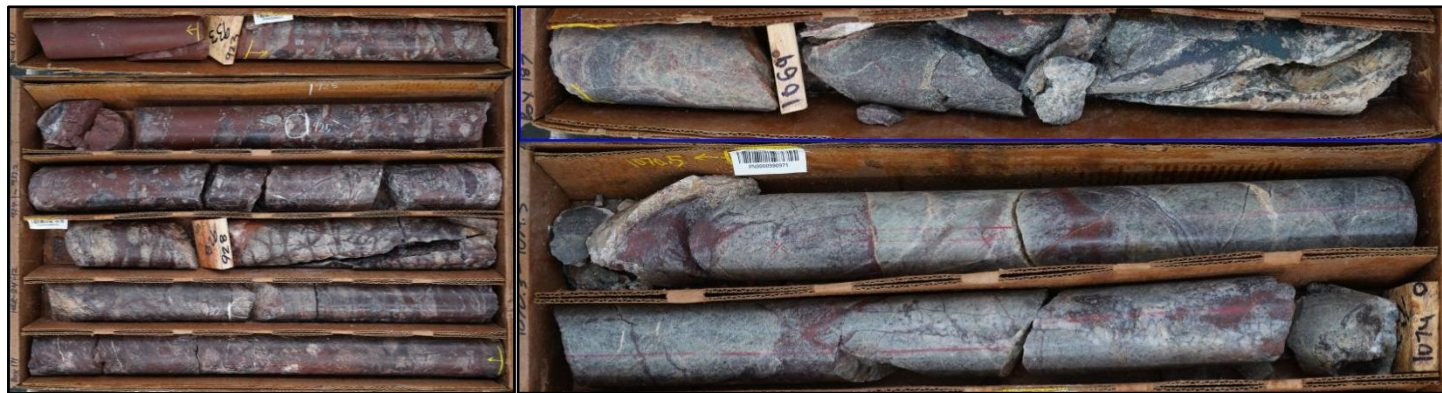
Drill hole 24-12 illustrating the typical transition from basal conglomerate, through leach cap, into the hypogene enrichment zone.
