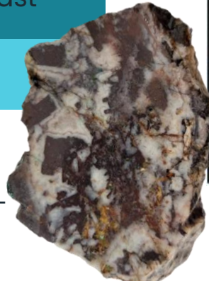
Hydrothermal Breccia with epithermal quartz textures – 1.2 g/t Au
